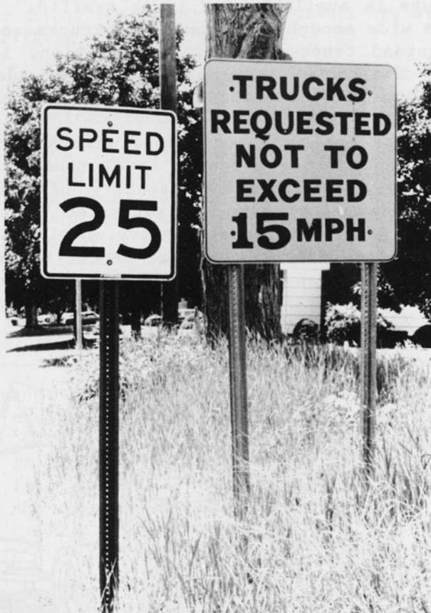
On this residential street leading to a factory, a suggested truck speed limit has been posted next to the official speed limit sign, MUCTD sign number R2-1.
