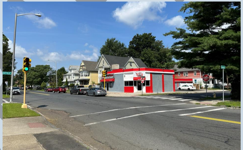
The corner of Wilbraham Road and Suffolk Street/ Colonial Avenue. This intersection has frequent pedestrian crossings, yet there is only one crosswalk across Wilbraham Road, with no pedestrian signals.
