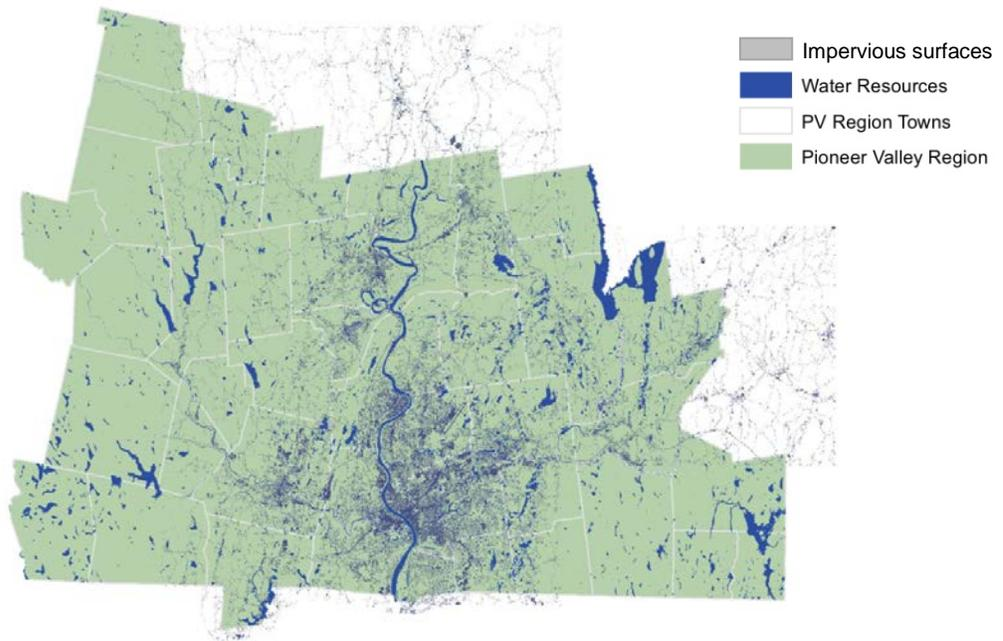
Source: MassGIS 2011. Impervious surfaces (shown in gray) are concentrated in urbanized areas. This increases the flood risk in these areas, as these surfaces impede the natural flow and infiltration of water. Concentrations of impervious surfaces also increase the Urban Heat Island effect.
