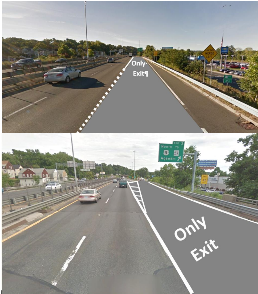
Figure 98 - Suggested "Exit Only" Markings on I-91 Southbound Before Exit 3 (© 2014 Google Earth Image).
