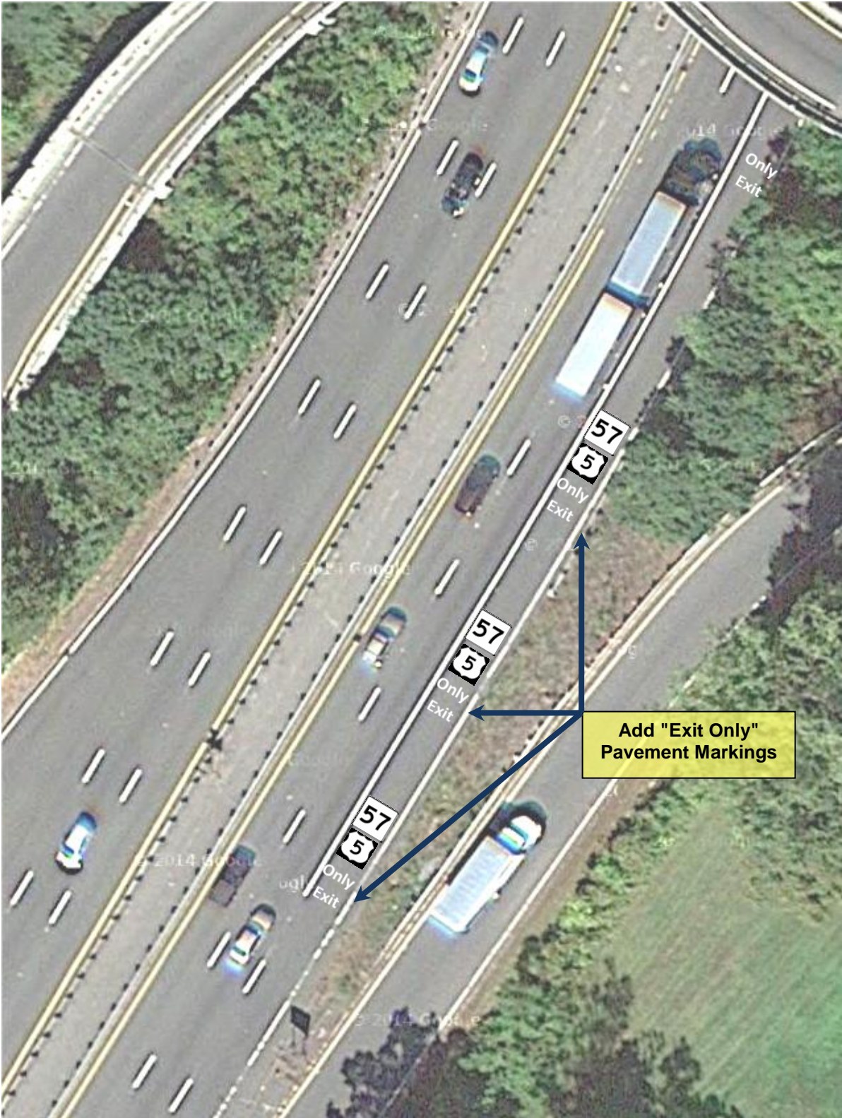
Figure 99 - Example of Pavement Marking to Designate Lane As "EXIT ONLY" Before Exit 3 on I-91 Northbound (Imagery ©2014 Terra Metrics, Map data © 2014 Google).
