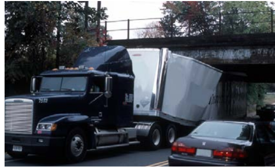
Truck stuck under a low clearance underpass in West Springfield
