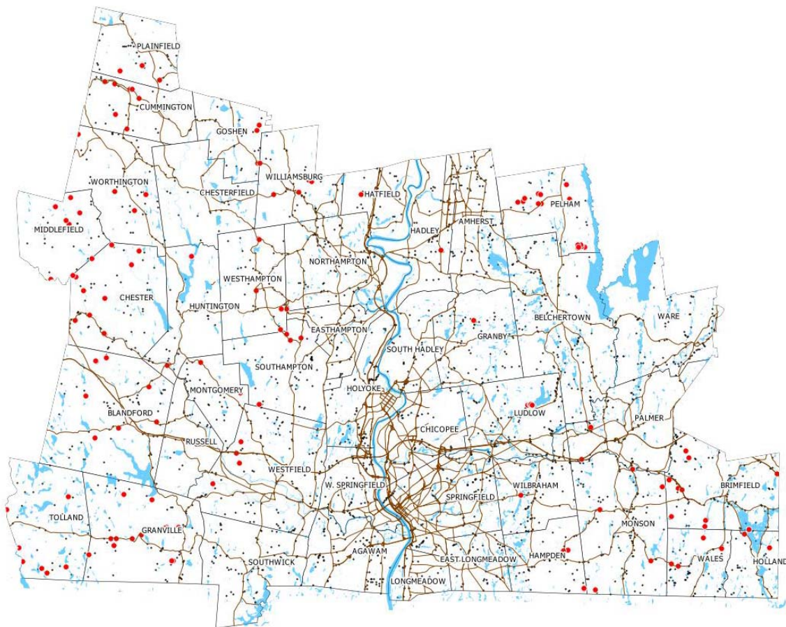
Figure 11-12 – Culverts for Roadway Crossings in the Pioneer Valley
