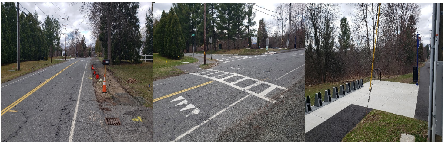
From Left: (i) Westbound approach of East Hadley Road, (ii) Crosswalk and Shark Teeth Yield markings, (iii) PVTA Bus Stop and Bike Racks located in the west of the crossing
