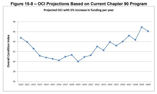
If level funded the Chapter 90 program will provide about \$450 million in funding to the PV Region. Based on our scenario the Chapter 90 program would need to experience a 5% per year increase in funding to maintain the current roadway condition. A 5% per year increase would result in a Chapter 90 invest in the PV Region of \$800 million over the next 20 years. This would result in a Chapter 90 program in line with the reports released by the MMA.
