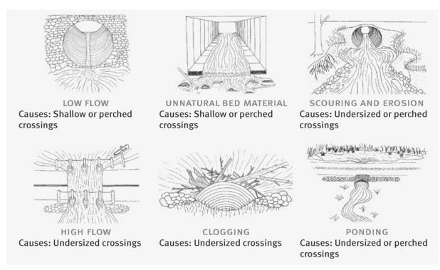
Common consequence of inadequately designed culverts and bridges are shown above.
