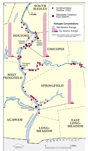
Figure 7-1: Combined Sewer Overflow Outlets and Wastewater Treatment Plants
