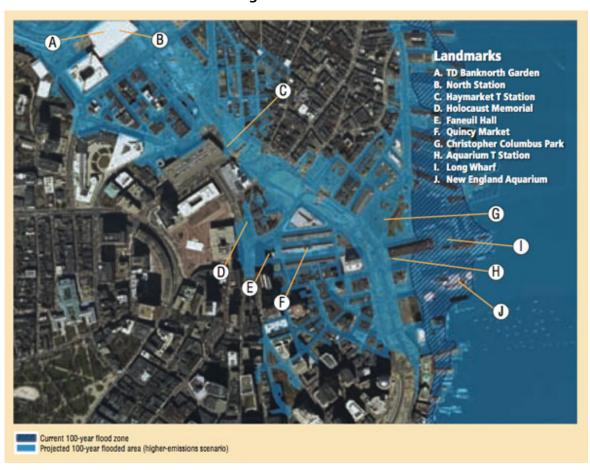
Figure 1-6: Projected Inundation of Boston Landmarks in a 100-year Flood
