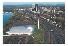
**Springfield I-91 Ramps:** While most sections of I-91 through the region are expected to be usable during floods because of the generally higher roadway elevation, a number of ramps in downtown Springfield are at a lower elevation and at risk of flooding from the Connecticut River. The most vulnerable ramps are Ramps 3 through 8, several seen in the northbound view in photo at left. This section of I-91 carries approximately 70,000 cars and trucks per day.
