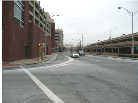
There are no parking lanes along this section of East Columbus Avenue. Bus operations to pick up passengers on this street configuration would cause vehicle backups and degrade traffic safety without significant roadway reconfiguration.
