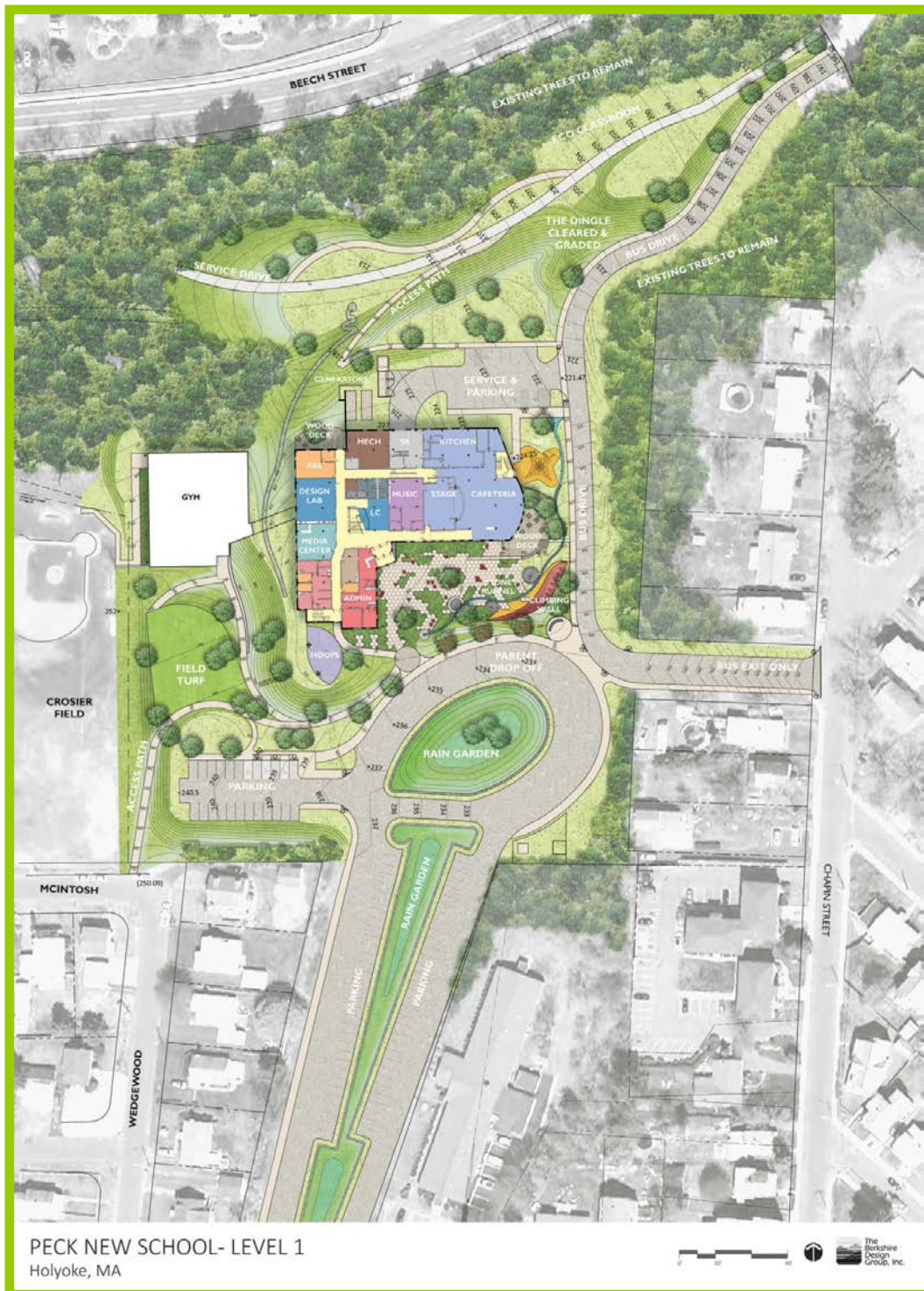
This conceptual design for the new Peck School features many green infrastructure stormwater systems integrated into the school's multi-purpose learning and play spaces. These include rain gardens, grass swales, and overall reduced impervious area.
