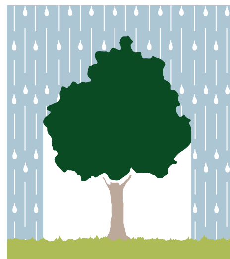
The surface area of leaves in the tree intercepts, absorbs, and slows down rainfall before hitting the ground, helping to reduce the flow of water draining toward the combined sewer system.
