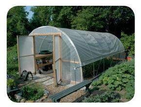
A **HOOP HOUSE** is an outdoor structure made of flexible PVC piping or other material covered with translucent plastic, constructed in a "half-round" or "hoop" shape, generally tall enough for a person to enter standing up.
