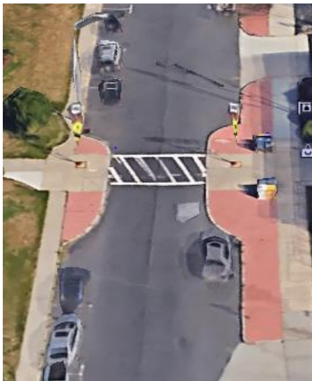
Figure 9 Example, from in front of the Post Office on Elm Street, of curb extensions with rapid flash beacons and crosswalk.
