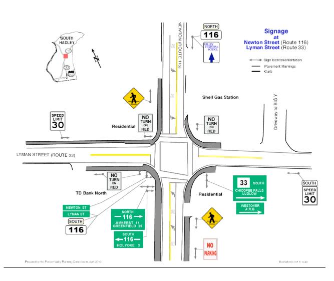
Figure 2: Pavement Markings and Signs at the Intersection
