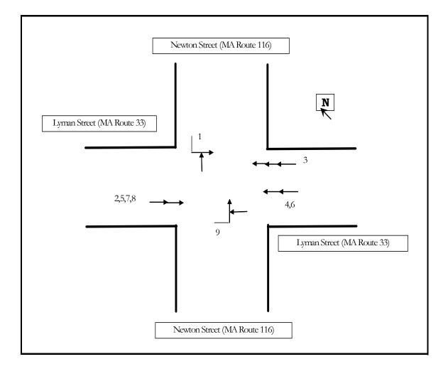
Figure 5: Collision Diagram
