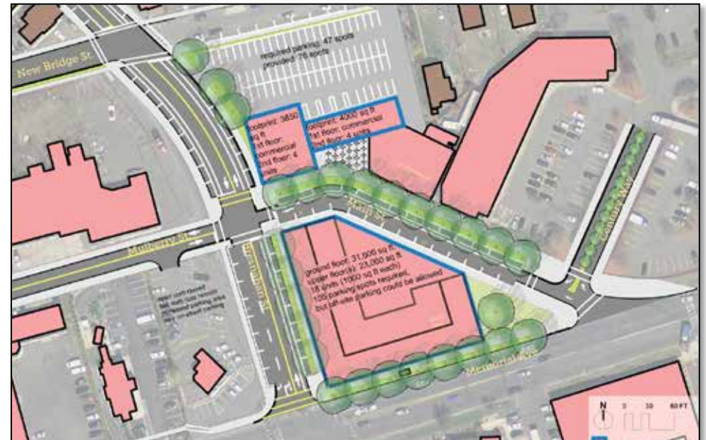
Redevelopment Concept. Narrow Main Street to create on-street parking. Install curbs and crosswalks. Realign the intersection of Main and Bresnahan to provide the opportunity to create a new development parcel and outdoor dining area. Enlarge 218 Main Street to increase taxable value.
